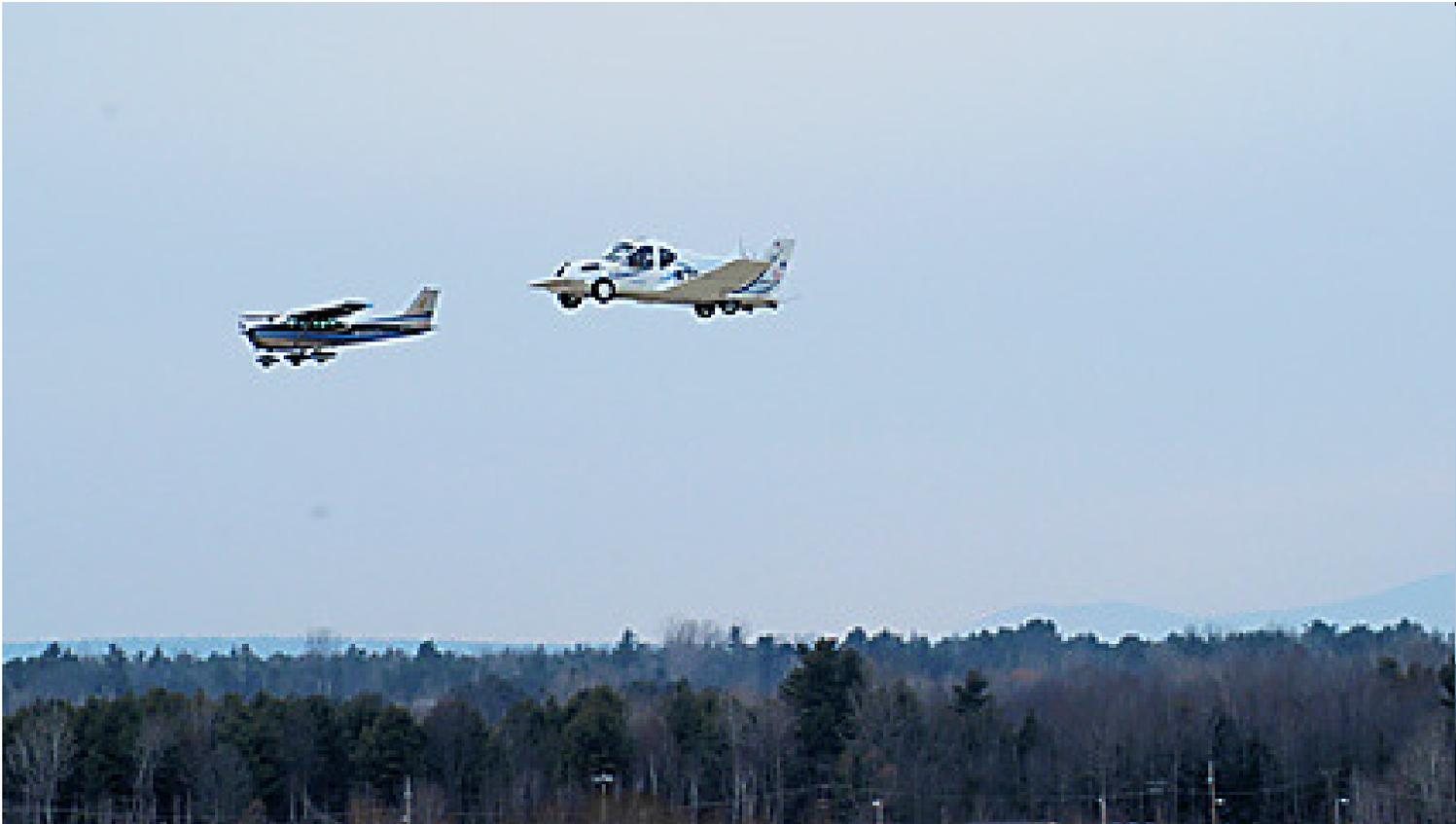
The Terrafugia Transition is a two-seater car that can convert from road to air in less than a minute, without the driver leaving the vehicle.
