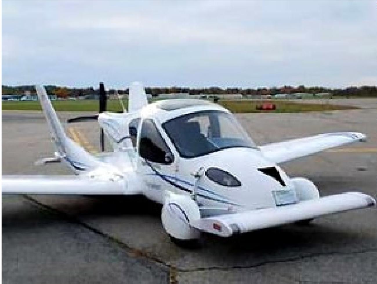
The Terrafugia Transition is a two-seater car that can convert from road to air in less than a minute, without the driver leaving the vehicle.
