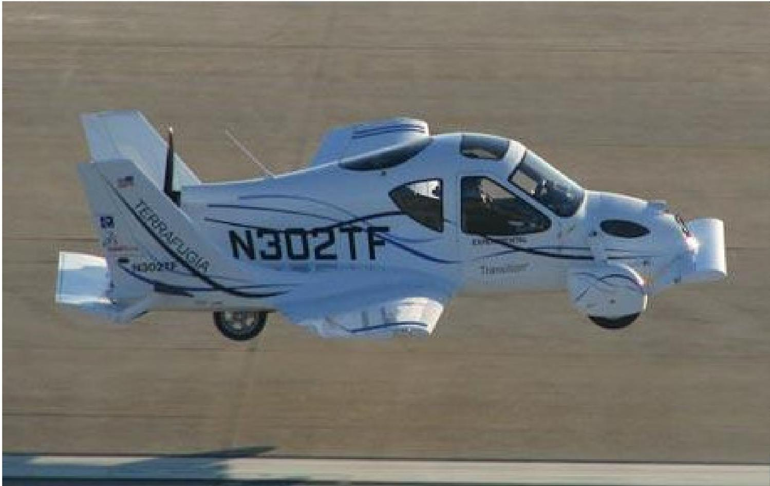
The Terrafugia Transition is a two-seater car that can convert from road to air in less than a minute, without the driver leaving the vehicle.
