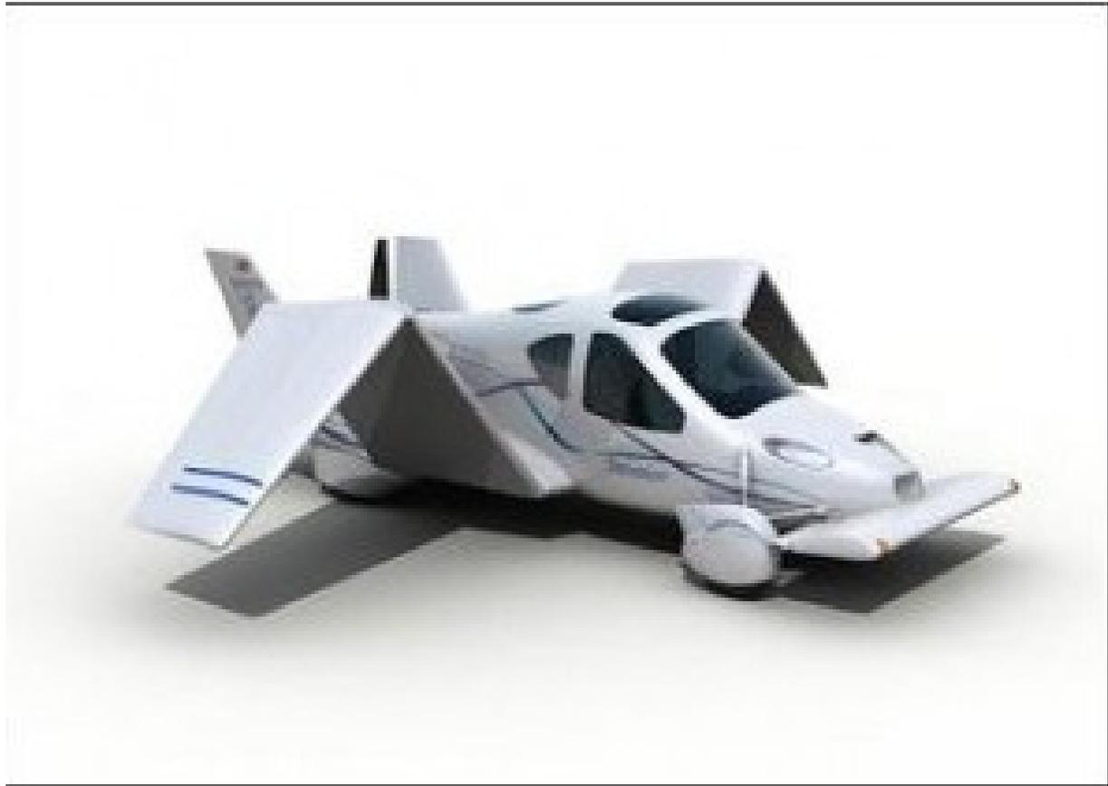
The Terrafugia Transition is a two-seater car that can convert from road to air in less than a minute, without the driver leaving the vehicle.
